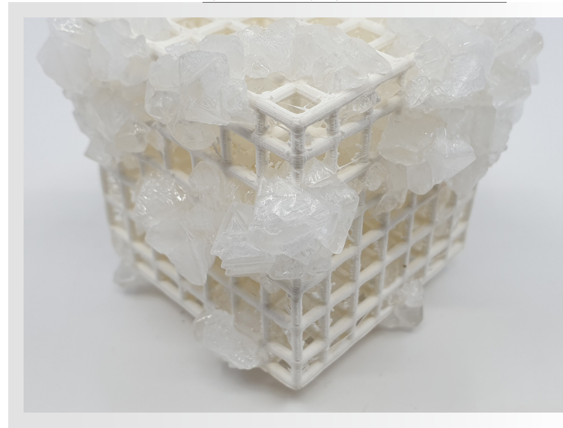
Figure 20 Successful crystal growth on 3D printed Lattice structure
