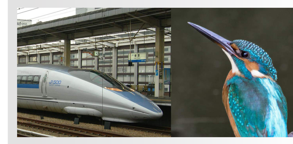
Figure 02 Biomimicry: Japanese bullet train mimicks kingfisher beak to reduce noise
